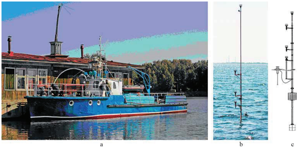
Fig. 3. a) Vessel on the Gorky reservoir. b) View of the operating state of the Froude buoy. c) Schematics of the Froude buoy.
