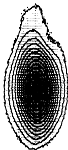
Fig. 7. Measured field distribution of one of output beams. Contour levels: 0.1, 0.2, ..., 0.9
