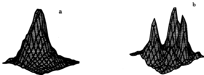
Fig. 4. Distribution of power flow density for a main (a) and cross-polarized (b) field components.
